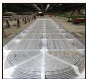
Fig-11. U Bend Storage Racks
