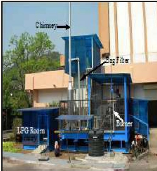
Fig.7 Simulated flue gas facility at EBC
