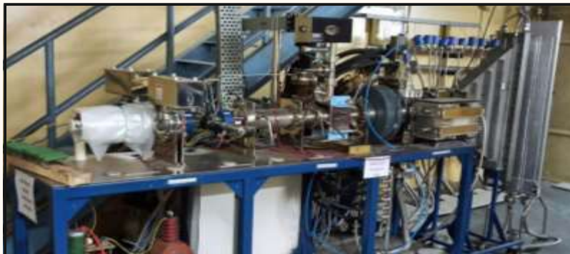
Fig.12 Photograph of X-band 6MeV LINAC Test setup
