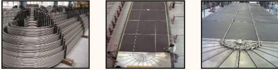
Fig-9. Surface Plate Gauge Block for U bend tubes
