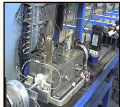
Fig-4. High speed Ultrasonic testing m/c.
